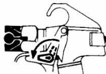
Trigger lock in locked position.
